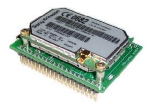
The GSM2-1A is a complete GSM/GPRS, which is ready to integrate into your application, it offers full standards multi-band GSM/GPRS Class 8.
